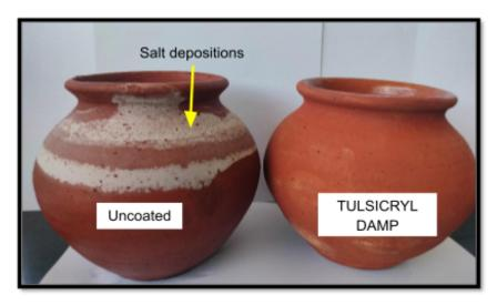
Furthermore, the top view confirms that the pot coated with **TULSICRYL DAMP 101** successfully retains the salt solution inside it, whereas water passes through the capillaries/channels and evaporates, leaving the salt deposits on the uncoated pot. Thus, coatings based on **TULSICRYL DAMP 101** are best suited in areas such as basement walls, driveways, or exterior coatings where water or moisture is always present.
